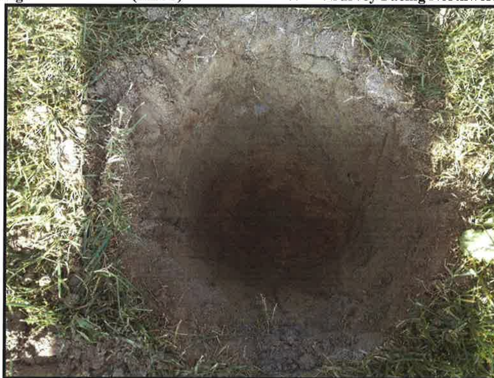
Image 4: West Parcel (Part 5) Typical Test Pit Profile
